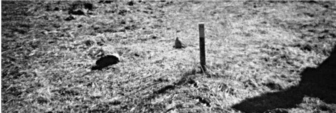
Now attach two tapes to the nail on the top of the peg (or survey arrow).
