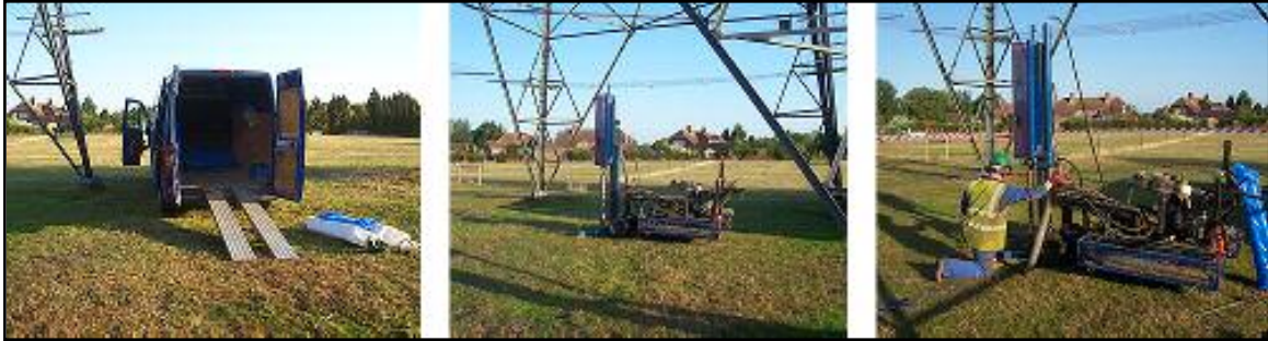
Figure 3: Window Sampler at work – Note the ability to be used even beneath a pylon.
