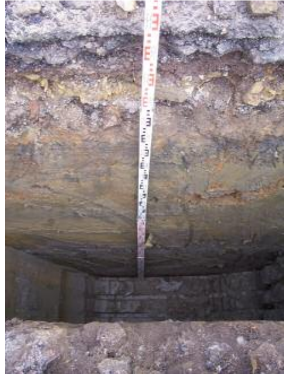
Figure 9: Test pit showing soil profiles.
