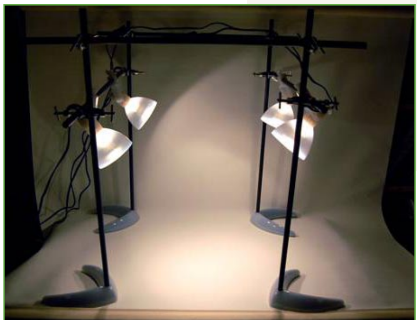
Figure 26. Simple home-made lighting rig for small object recording
