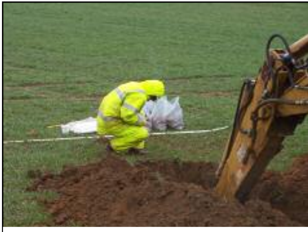
Figure 2: Engineer marking samples from test pit.
